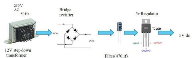
Fig. 6. Regulated power supply
