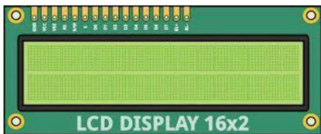
Fig.4. LCD Display
