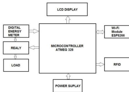
**Fig. 1** Block diagram of proposed prototype smart energy meter
